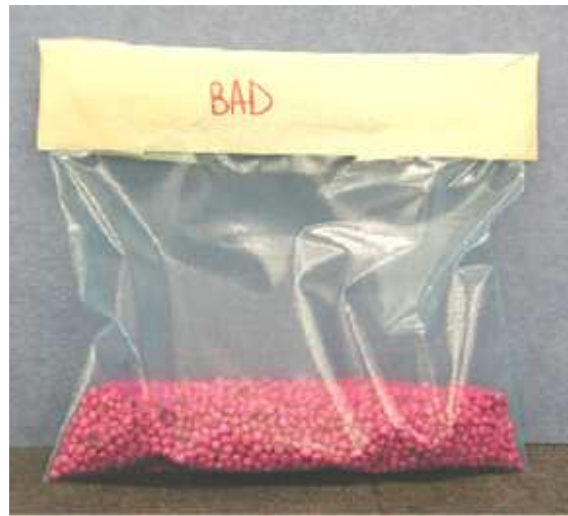
Figure 1b: Improper sample for moisture, not enough seed and air not removed from bag.
